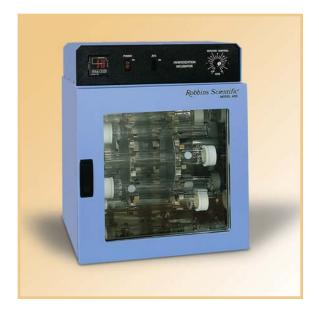
The Model 400 Hybridization Incubator is uniquely designed with a passive heating system to provide precisely controlled temperatures within the incubator chamber. Sturdy rubber strips with embedded heating wires surround and heat the stainless steel chamber. The resulting warm air within the chamber is then circulated through movement of the rotator to ensure temperature uniformity. A precision controller regulates the temperature to
